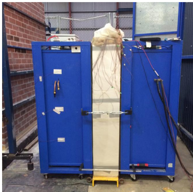
Figure 33. Rammed earth wall undergoing tests in the thermal hot box (Netherton, 2015).
