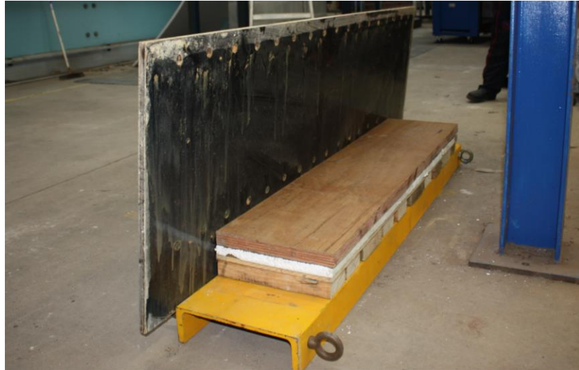
Figure 28. Rammed earth wall support and packing beam (Netherton, 2015).
